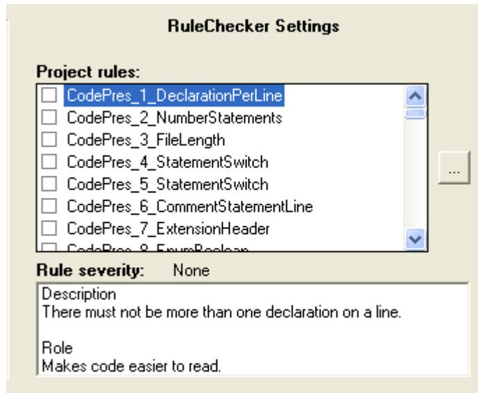
16. For the purpose of the example, just uncheck the rules: **Complexity\_14\_InclusionLevel** and **ControlFlow\_4\_ThenElse**.
