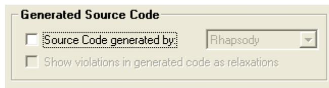
**Source Code generated by:** when the box is checked, allows to specify the tool (e.g. *Kalimetrix Rhapsody*) used to generate all or part of the source code under analysis. Thus, *Logiscope RuleChecker* will not considered the violations found in the generated code. For more details, please refer to section 1.5.8.
