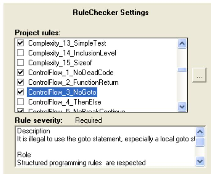
The description of the selected rule and the rule severity are displayed in the bottom pane.
