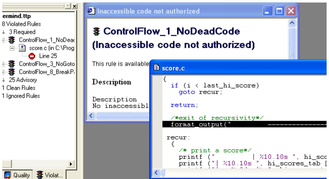
Indeed this is dead code: i.e. some executable statements that can not be executed. The *Rational Logiscope RuleChecker* module definitively improves efficiency of the code reviewing process.
