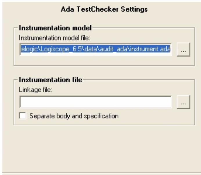
The **Instrumentation model** is an Ada file to be used as a template to generate the instrumentation file when building the instrumented executable (see next section).
