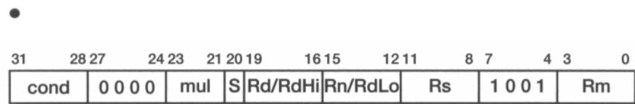
**Figure 5.7** Multiply instruction binary encoding.
